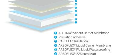
ARBOFLEX® PU Liquid Waterproofing
