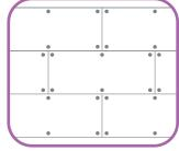
corrugations. All board joints should be fully supported by the deck.
