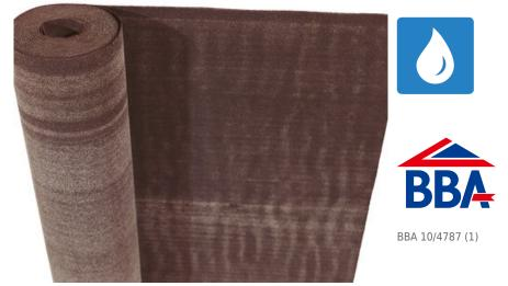
GLASDAN 30 AP ELAST. (7,5 M) is a waterproofing bituminous sheet with non self-protected surface of 3.0 kg/m<sup>2</sup>, LBM-30-FV. Composed of a fibreglass reinforcement and covered on both sides with SBS modified bitumen mastic. Membrane with an upper surface finish of sand and a lower surface finish of polyethylene film.
